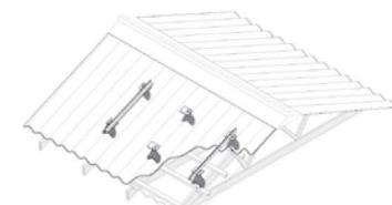
All solar collectors must be fixed at no less than 4 points.
